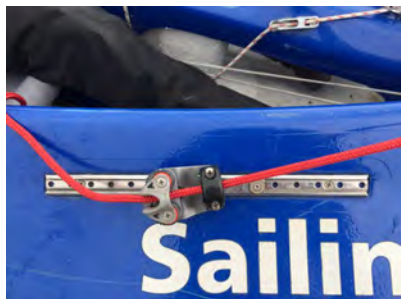
Jib sheet cleat and track- lift the pin to slide the cleat along the track
