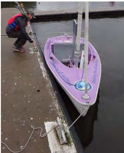
Tie up front and back to the cleats fixed on the pontoon
