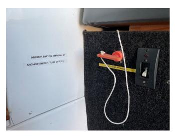
Turn ANCHOR WINDLASS OFF. Power switch for anchor windlass is on the side of the bench seat. Turn red leaver to left and flick switch to power off. (Image shows off position).
