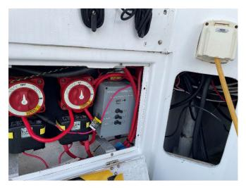
Flick on three House Battery switches to the RIGHT for OFF: Toilet & Cabin, Cockpit, Helm.
