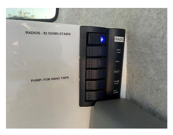
Turn on RADIO. This powers the two downstairs VHF radios, accessed from inside the cabin or outside the cabin with the additional handsets.
