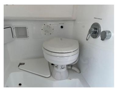
The HEAD is flushed by pressing the black button behind the toilet. It will take a few seconds before water comes through.
